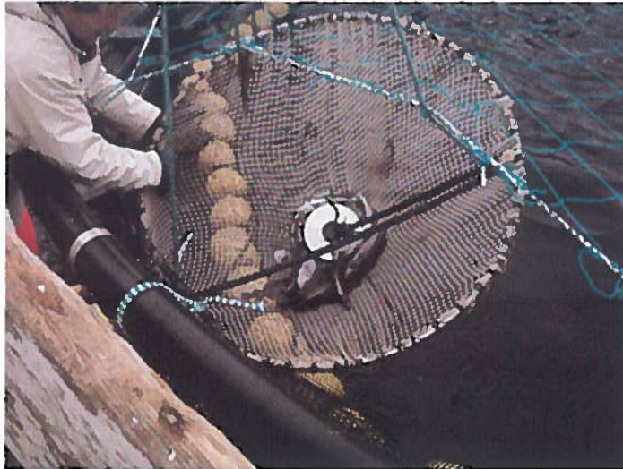
Figure 4. A net ring with weight is at the bottom of the cage. Dead fish will sink to the bottom and can be pulled up and collected (photo: Thorleifur Agustsson).
